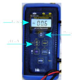
Power button in bottom row. Turns off automatically if idle for several minutes.
