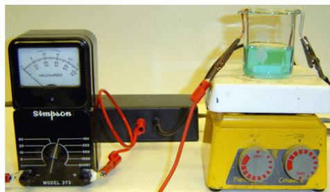
**Figure 5** Electrodeposition Cell Set-up
